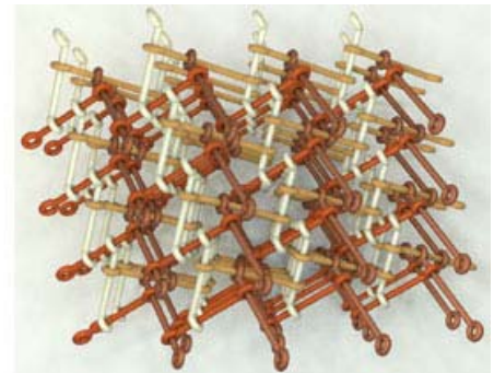
Figure 35: Space frame grid F.
